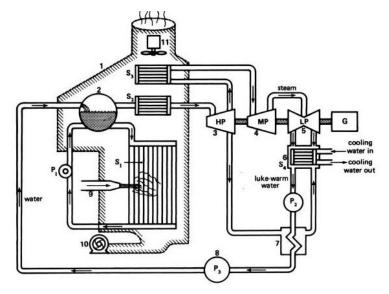
The super heated steam carries the stored energy to the steam turbine.
